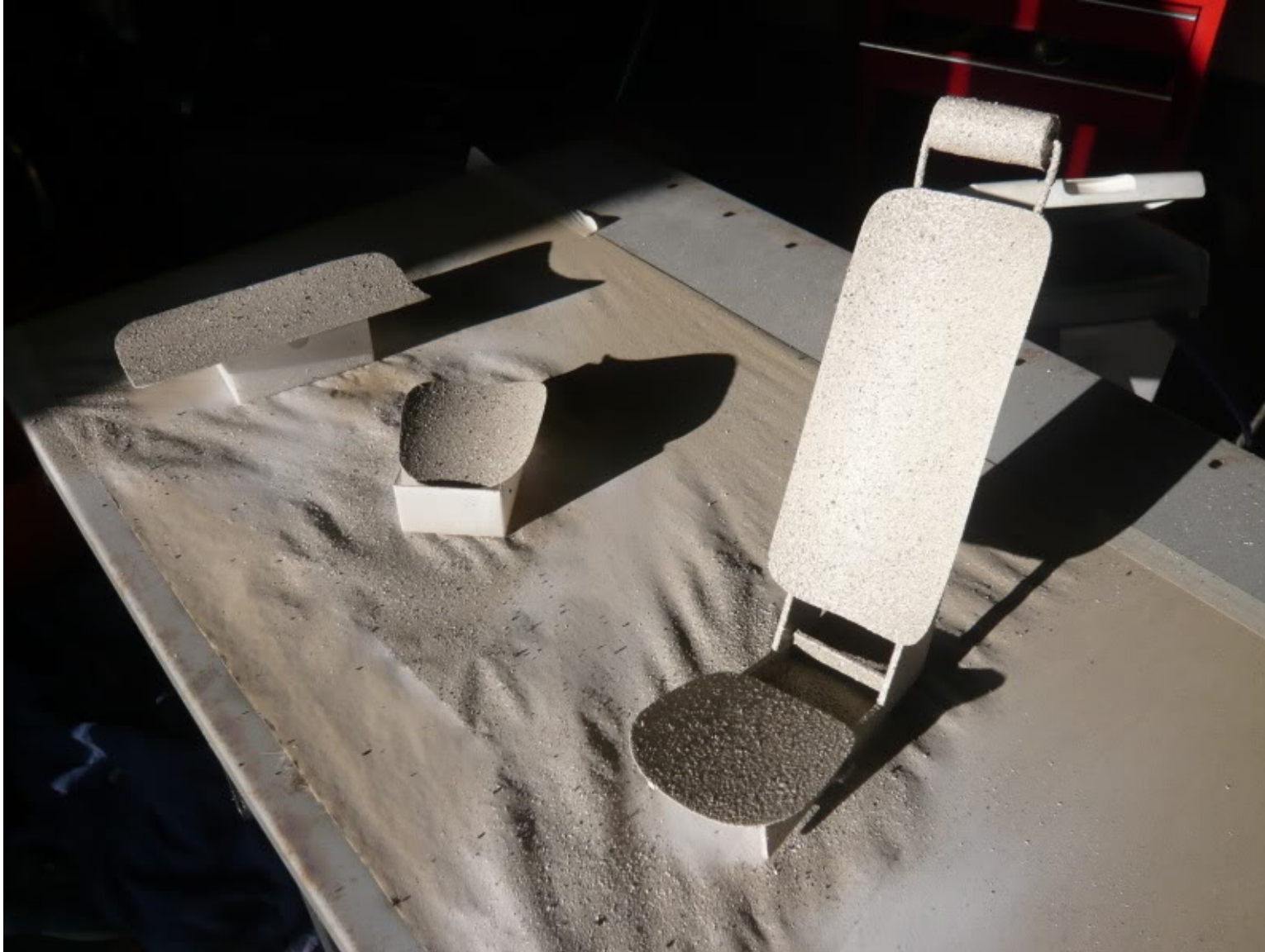
The front and rear instrument binnacles I made by carving lumps of foam to (about!) the right shape and then glassing them. I drew the panels themselves by scaling photographs and doing a CAD drawing. Luckily my local school has a laser cutter that I can use so they were cut from perspex direct from the CAD drawing. The instrument jewels are thinner so that they give a 3D effect. The instruments themselves are just prints from photographs stuck to the back of the lenses. Unfortunately I couldn't find any really high quality ones (without paying!) so they are a little blurry.
