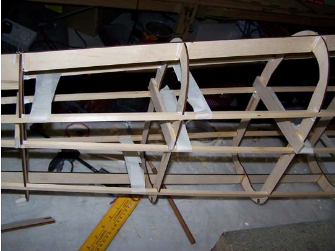
and a few cross pieces added in to help reduce twisting
