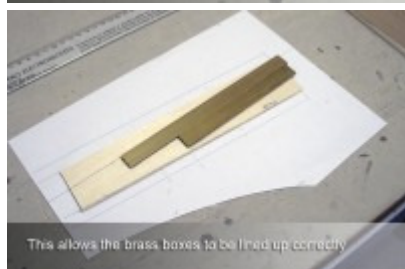
Drawing & component parts of the joiner box
