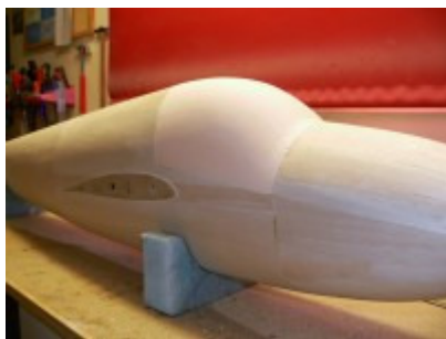
The raw canopy plug finish sanded.
