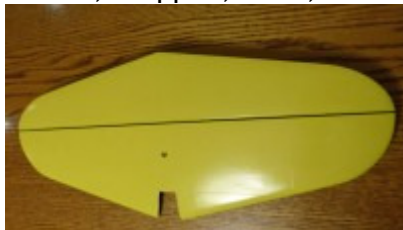
Tailplane stripped, lined, resprayed and hinged.
