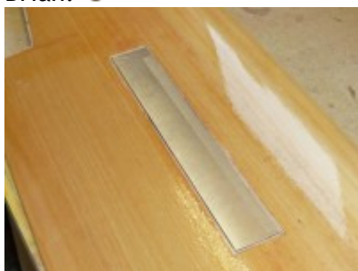
Blade in place flush with wing surface.
