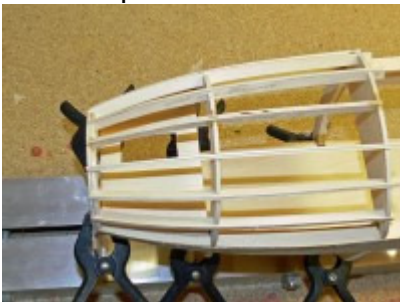
The tray added to the nose to provide a home for the aerotow release servo.
