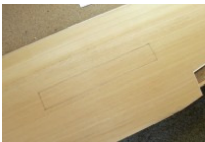
Scale position of the top spoiler box marked out.
