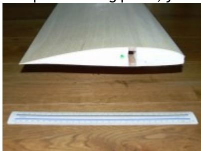
The wing root showing the HQ3.5/12 profile, the wiring conduit and the spruce spars.
