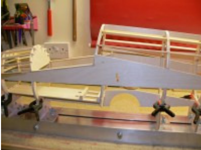
Cockpit area and center section all joined together by the side frames.
