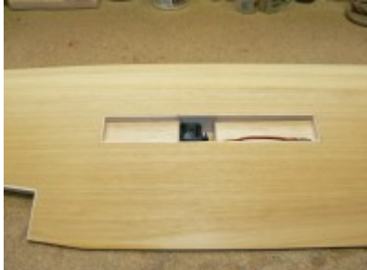
Spoiler box excavated and lined.
