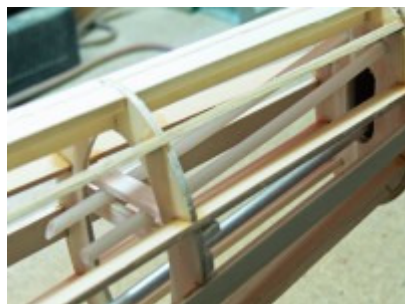
The pull-pull cable conduits firmly located in the rear fuselage.
