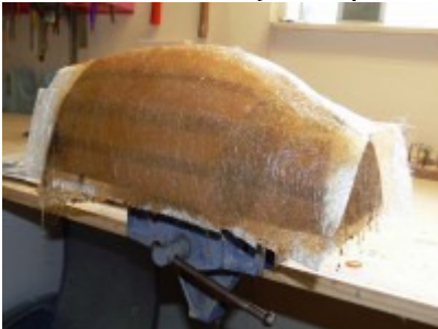
The chopped strand mat and resin in place.
