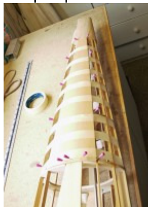
A start made on the aft fuselage 1/8 balsa sheeting.
