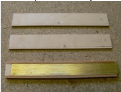
The brass box glued to the front face, the top and bottom rails and filler.
