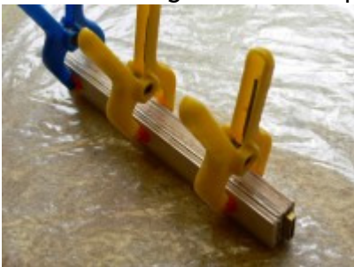
The filler piece which provides a stagger on the boxes glued in place.
