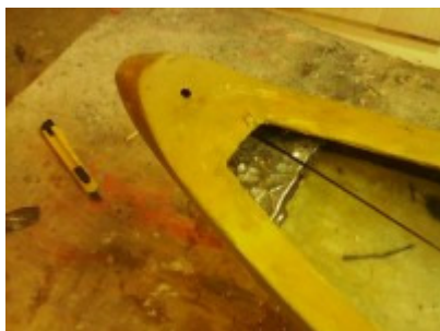
Lead cast for nose 1.2 kg.
