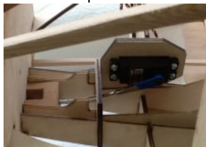
Release in closed position
