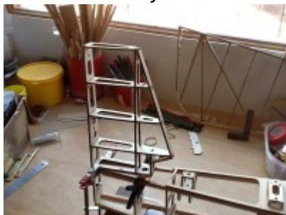
Fin assembly in place
