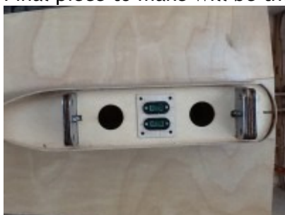
Wing servo MPX sockets in top of pylon
