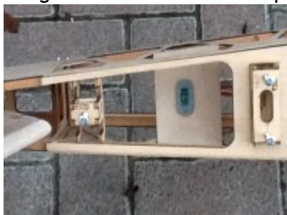
Tailplane servos MPX socket
