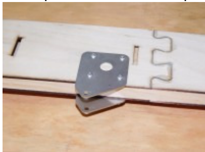
Strut attachment point
