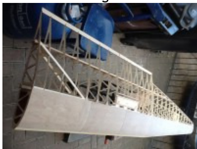
LE fitted awaiting profiling
