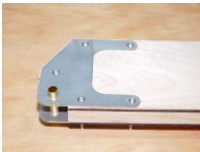
Main spar_Fuz attachment point
