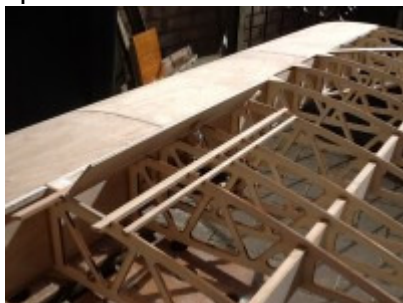
Spoiler blade core open
