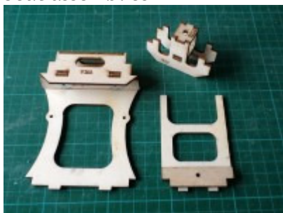
Tailplane fixing assemblies
