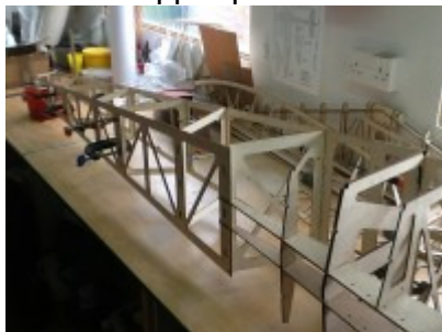
Rear fuselage formers being fitted
