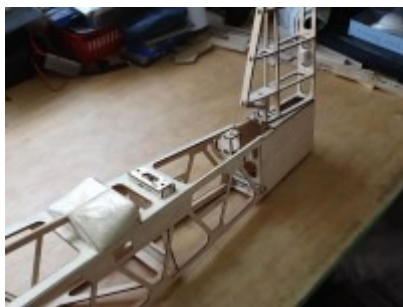
Rear fuselage fairing
