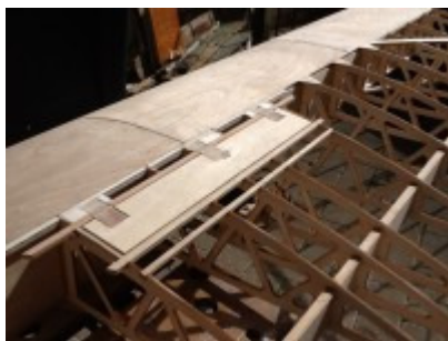
Spoiler blade core closed
