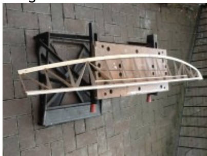
Aileron with 1st LE sheet
