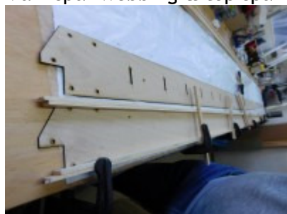
Main spar webbing & lower spar strip glued
