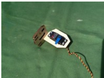
F1A with aerotow servo mount
