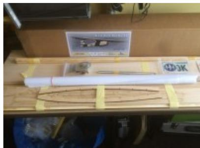
I started preparing a desk for rudder and elevator construction. The plan is covered with the thermal lamination film for documents lamination and lightly sparkled
