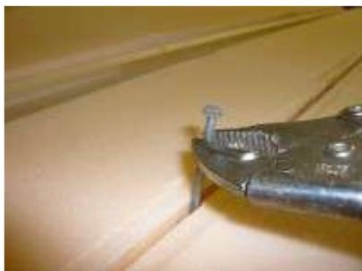
Cut the shear web slot using a heated up nail melting right down to the fully cured spar cap, then put in the rammed shear web, pooled it all with thickened epoxy and then repeated the multiple lengths of carbon rovings for the other side's spar cap.
