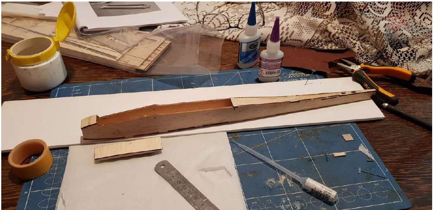
6: Fuselage, basically framed up.
