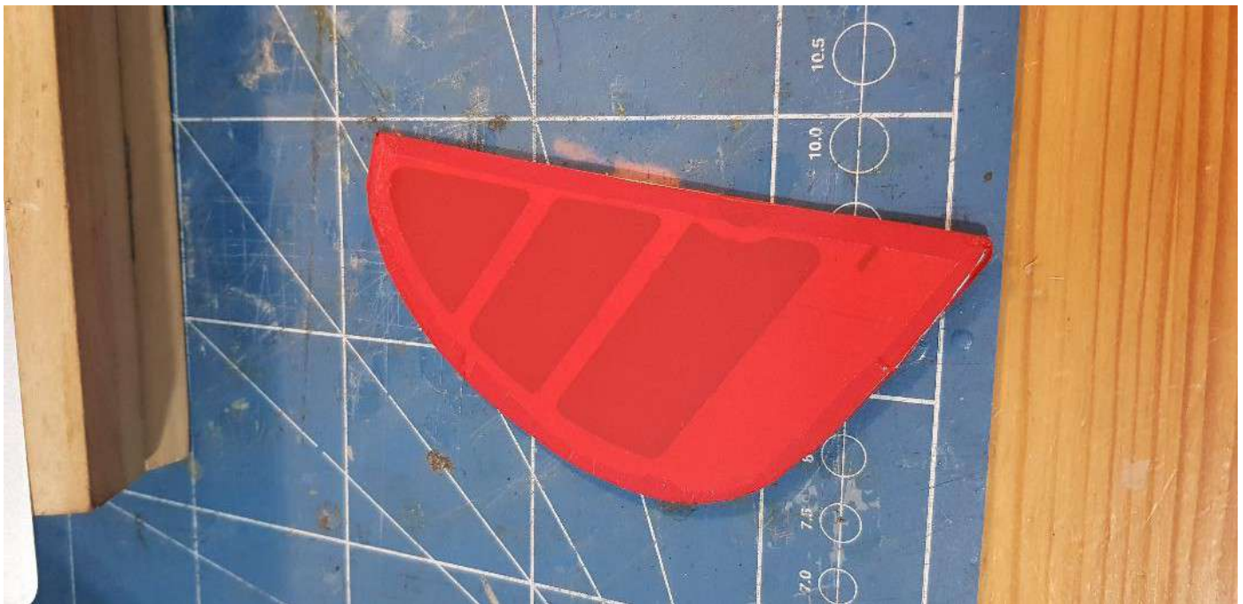
26, 27: First experiment; covering the rudder in one piece. Do-able.
