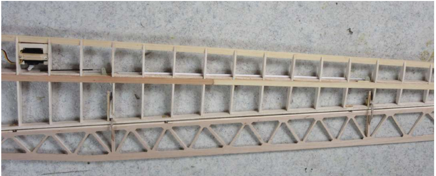
26: Aileron actuation in one picture seen from below.
