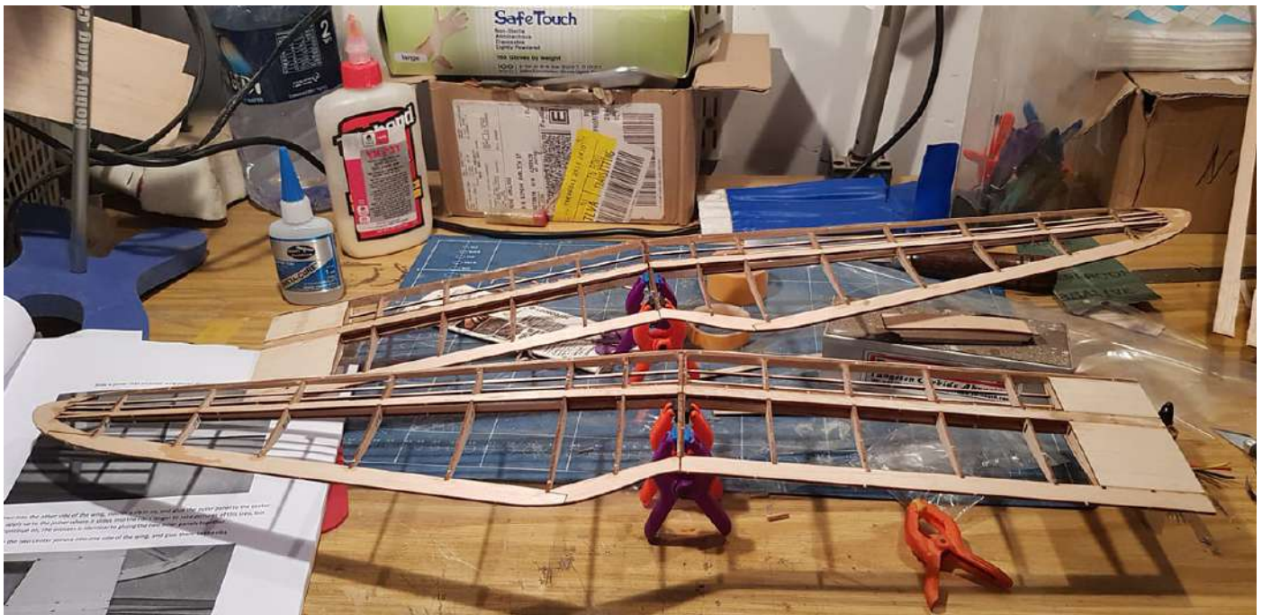
22, 23: Joining the wing panels.
