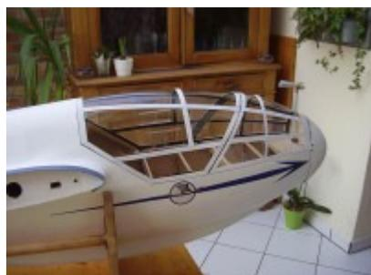
Canopy is completed with ABS white strips, an army of little screws or rivets is to come
