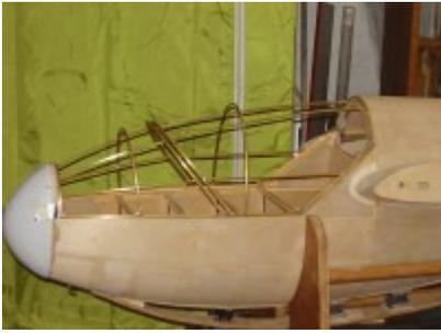
I have no other pictures. This is the first step. Soldered 4mm brass tube, then I add ( with neoprène contact glue) some 0,3 aluminium strips(10mm wide) then 0,8mm wood strips (6mm wide) to accept the transparent material depth . All pieces of glass are cut separately) then I'll add another 0,3 mm aluminium strips over( 10mm wide glued and fixed with screws or rivets)
