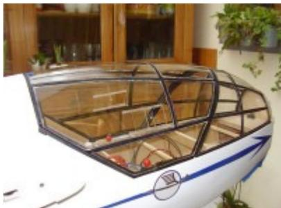
Work is coming to its end on the canopy. All the transparent panels are cut and glued separately. A white strip to be fixed over. The home-made "ventilators" allow acces to the lock system.
