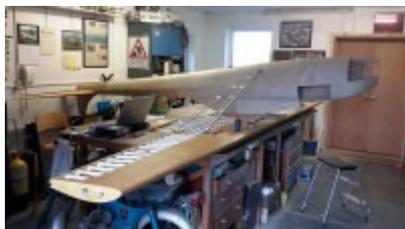
With the poor flying weather progress has been good on the Wien. Fuz sheeting almost complete and now working on the wing struts.
