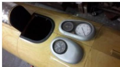
Another poor day for flying so in the workshop making the instruments and housings for the Wien instruments. The housings were vac formed to simulate the formed aluminium of the original and the instruments were made up of all individual parts including individual hands for the dials.....Yes, I know I should get out more !
