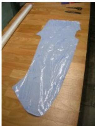
..made a small template to cut the glass fiber...
