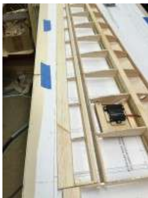
aileron cut and servo mounted
