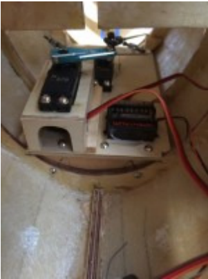
Front view showing the elevator servo.
