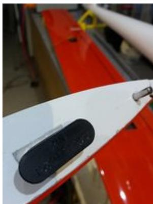
I am the world's worst solderer and I did not like the idea of soldering up a 9 pin din plug and socket so I made my own from 2mm bullet connectors. These are permanently fixed in the wing roots and make automatic connection when the wings are put together. The advantage of the 2mm bullets is that they have a much longer insertion than the din plugs, some 9mm compared with just 2mm for the dins.
