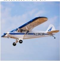
For electric flight they recommend 5s or 6s LiPo. This would be OK for scale flight but for towing or frolicking around I'd suggest 8s. It's always more efficient to get the power from big volts than big amps. 8s would allow you 2kW with less than 70A current.
