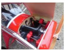
I spent a day making a perfectly acceptable plywood motor mount and battery box, found it weighed 500g, then binned it and moulded a 100g version from carbon cloth. Much more blingy don't you think? The radio batteries (2 x 2400mAh NiMh) are slung below each LiPo on trays either side of the motor.
