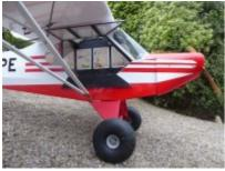
Having all the powertrain in the cowl means the cabin is embarrassingly empty! There's just a receiver lurking in the bottom plus a rudder servo and bellcrank driving a close loop system. The kit recommends putting the rudder servo in the tail but my way is lighter and scale. Mind you, I did swallow hard and screw the elevator servos into the tail. Ugh! Practical, but so vulgar!
