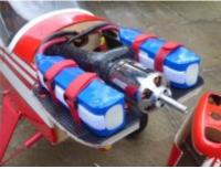
I settled on a 10s LiPo 4500mAh battery, (made from 2 x 5s 4,500mAh batteries in series), controlled by a Hobbywing 100A HV ESC, powering a Turnigy 63-74 149V motor spinning a 24x10 prop. The target was 70W/lb max, so 2100W at an estimated AUW of 30lbs, and 6 mins + duration.
