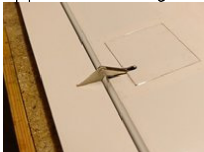
Pushrod / horn detail.
