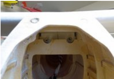
View from the cockpit with the wing screwed in place.
