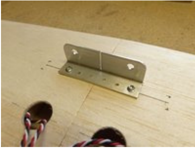
Wing Joiner bracket screwed to the wing.
