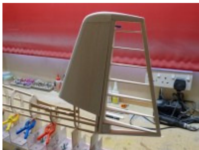
A trial fit of the completed fin.
