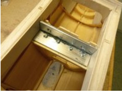
Wing Joiner bracket screwed into the fuselage.
