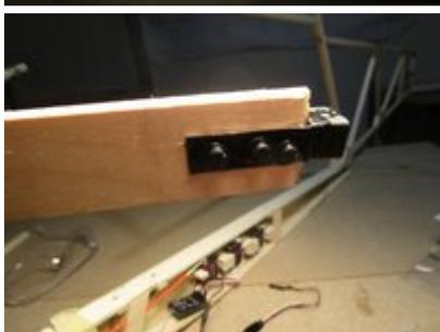
The worth point is that, I used carbon rod of 1mm diam. as dowels to enhance the joints.
