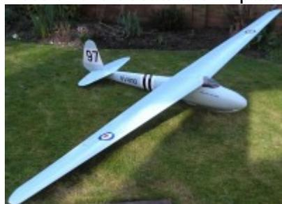
Remaining decals will be applied in next couple of days, together with another 1.5lbs of lead or so, depending on battery used.
