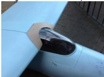
Underside of fairing coated with epoxy to try to lock in the curvature aft of the canopy. More shots of this to follow once fully cured.
