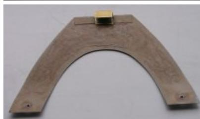
I think that I might go for a layer of lightweight glass cloth on the top down to just before where the L/E curvature starts as the thin internal epoxy layer hasn't done anything more than slightly stiffen the assembly.
