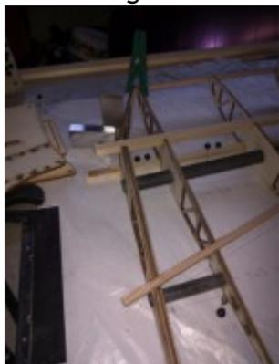
Initial wing root assembly with carbon tubes.
