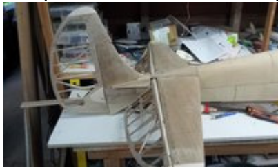
tail bits are made and test fitted
