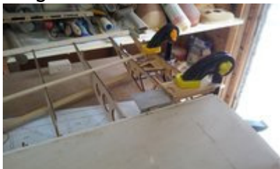
securing wing inner section to board
