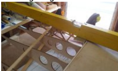
checking if wing is level
