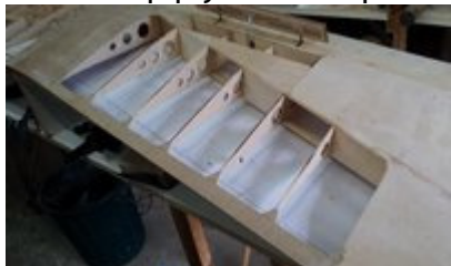
T/E planked at inner section
