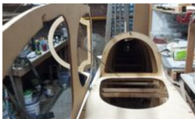
a piano wire restrict opening angle of canopy
