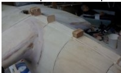
skid attachment blocks to extended fuse formers
