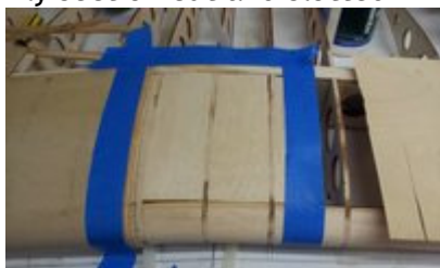
Ply section cut and slotted
