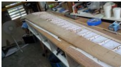
Front planking completed
