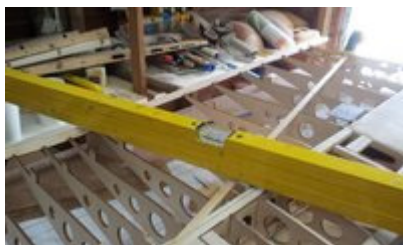
checking if wing is level
