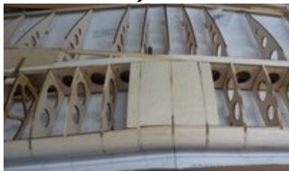
6mm balsa sheest between ribs at gull radius
