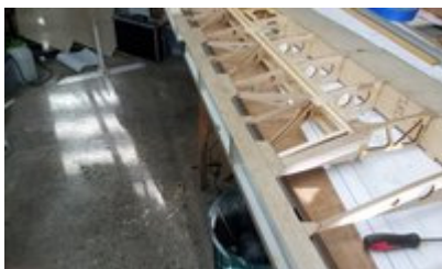
first aileron T/E planking fitted
