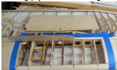
second sheet prepared glue area taped.
