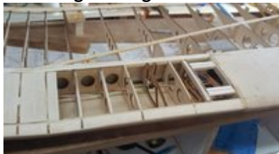
servo wire harness fitted
