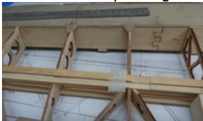
top spars recessed for hinges
