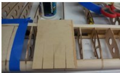
Ply section cut and slotted
