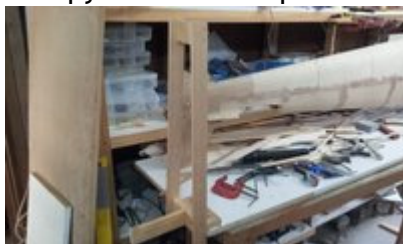
temporary frame for fitting canopy
