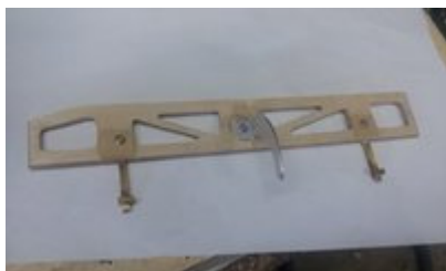
servo screws added from underneath
