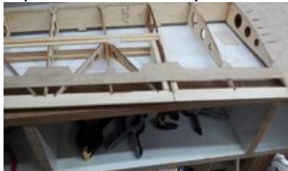
T/E planking prepared for aileron
