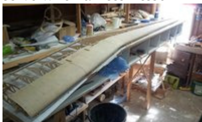
Front planking completed
