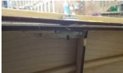
a piano wire restrict opening angle of canopy
