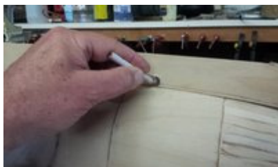
rolling washer with pencil to get a contour
