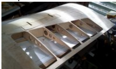
top of inner section planked with all bits and pieces
