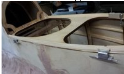
canopy frame in place and hinged
