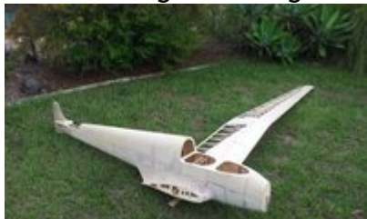
fuse and wing mated together
