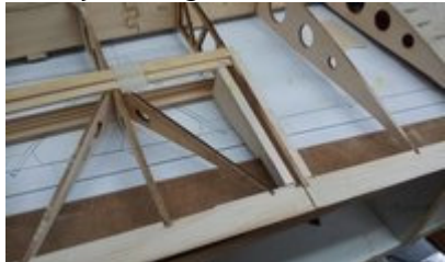
aileron diagonal ribs fitted
