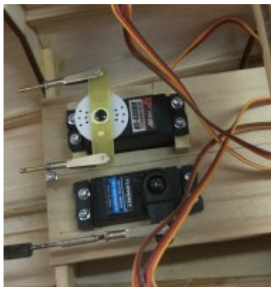
Revised fuselage servos
