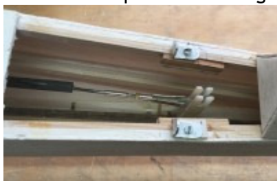
Elevator crank connection
