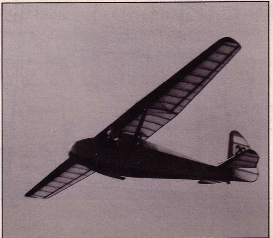
Gentle stall characteristics, no adverse yaw with ailerons and a light wing loading all help make the Pegasus a delight to fly.
