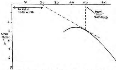
Along the airspeed axis lay off the amount of the headwind component; from this point reached, draw a new tangent to the polar curve; the point where it touches the curve corresponds to the "best" airspeed for those conditions.
