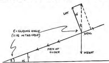
flattest when the ratio L/D is a maximum. This maximum corresponds to a definite angle of attack (see Appendix). Therefore in order to cover the largest amount of ground, in still air, we must fly at this angle of attack (about 7° for the Olympia).
