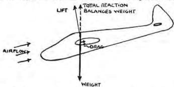
through the centre of gravity. (The centre of gravity is that point about which the aircraft, if placed on a pivot, would be perfectly balanced.)
