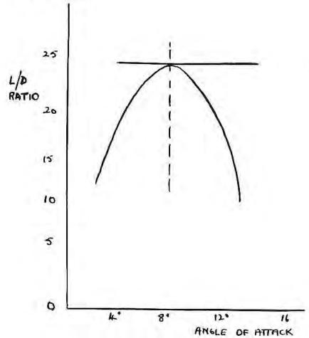
It was shown on page 13 that the angle of glide (in still air) is flattest when the ratio L/D is a maximum. Observe that this occurs at an angle of attack of about 7°; at normal loading this corresponds to an airspeed of about 45 m.p.h. (39 Knots).
