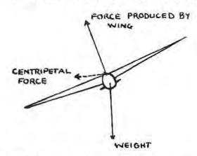
of the centripetal force required varies with the rate of turn and with the airspeed.
