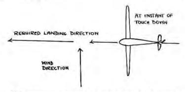
This counteracts any strain the touch-down might cause the undercarriage, by swinging the aircraft in line with the direction of motion; if this is done at the correct moment, the aircraft will touch down before the flight path has altered.
