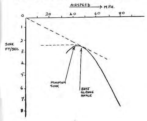
The graph obtained for a given glider is known as its "polar curve" and is of the type shown; this curve was obtained for the Olympia at 630 lb. all up weight.
