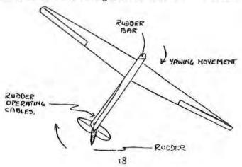
the rudder bar. When the rudder bar is pushed forward by the right foot, the rudder moves out to the right-hand side, and therefore is reacted on by the airflow. As a result the tail of the aircraft moves round to the left, the aircraft pivoting on the centre of gravity; the nose thus moves in the direction of the right wing-tip. When the rudder bar is pushed to the left the reverse happens, the nose moving in the direction of the left wing-tip. These movements are in the "yawing plane."
