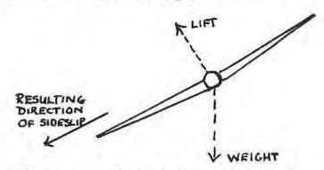
The steeper the angle of bank, the greater will be the sideways component of the motion. However, the sideslip is an unnatural condition of flight, both the lateral stability and the weathercock stability trying to prevent it. The lateral stability tends to level the wings again, and the weathercock stability tends to convert the sideslip into a turn.
