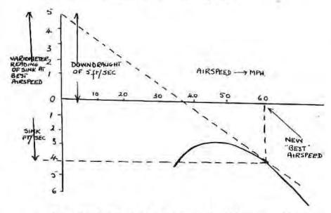
A rough rule indicates that the speed should be increased by 3 m.p.h. above 45 m.p.h. for each 1 ft./sec. increase in sink; thus in a 5ft./sec. downdraught, the Olympia should be flown at 60 m.p.h. (52 Knots).
