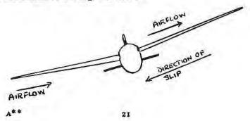
In consequence the lower wing meets the sideways component of the airflow at a greater angle of attack than the upper wing, and will therefore have more lift. This greater lift restores the aircraft to the normal level position.
