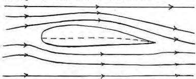
The result is that the air passing under the aerofoil increases in pressure and exerts an upward force on it, while the pressure of air passing over the top of the aerofoil is reduced and this exerts an upwards sucking effect. Thus both the air passing over and the air passing under have a lifting action.
