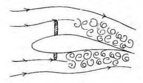
They are of robust construction and may be used to limit the diving speed of a glider to a safe maximum. They are also used in the same way as spoilers to assist in controlling the approach. Their effects are:
