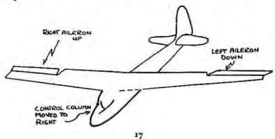
Movement of the stick to the left raises the left aileron and depresses the right aileron. Thus the left aileron presents a reduced angle of attack to the airflow, and therefore gives less lift; the right aileron, having been lowered, presents an increased angle of attack and hence gives more lift.
