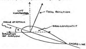
In the diagram here we represent each force by a line in the direction in which the force is working. The length of the line respresents the strength of the force involved.
