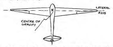
Remember.—No matter what the attitude of the aircraft is in relation to the ground, the controls always have the same primary effect on the aircraft (unless it is stalled). The ailcrons give control in the rolling plane, the elevators in the pitching plane and the rudder in the yawing plane. These planes are referred to the aircraft and not to the earth.
