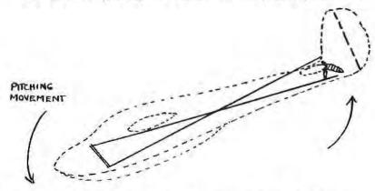
tail. Similarly when the stick is moved forward the elevators are depressed and the nose goes down. The elevators thus
