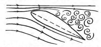
It is when the air over the aerofoil is in this turbulent state that the aerofoil is said to be stalled. Stalling occurs when the angle of attack is increased beyond the "critical angle" or "stalling angle," or "angle of maximum lift." The value of this angle depends on the design of the particular aerofoil. Stalling always occurs when the angle of the aerofoil to the airflow is increased beyond this value, and it cannot occur unless the angle is so increased.
