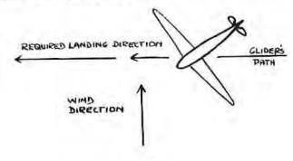
Just before touching down, rudder should be applied in the direction of drift :-
