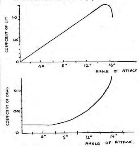
In order to make simple calculations using the lift and drag formulae, the correct values of the coefficients can be extracted from the above graphs.
