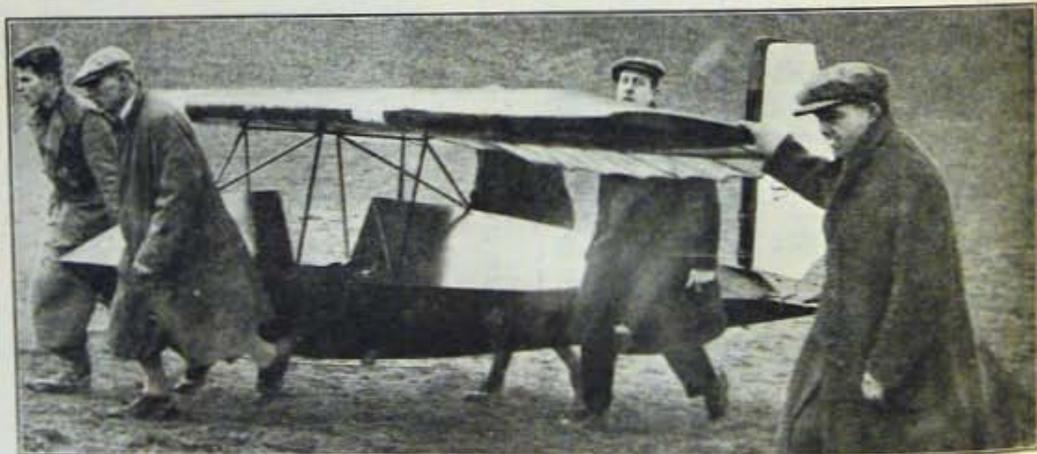
PORTABILITY.—The Brant "Scud." Mr. Baynes, its designer, nearest the camera on the left, carrying his baby. The diamond cross-section facilitates carriage.
